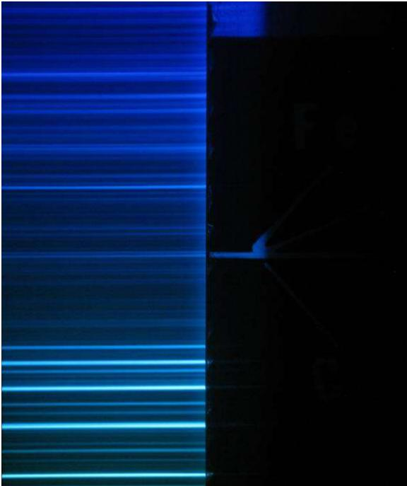
The gold line at left is now easily seen and aligns with the film gold line at right. The other visible blue lines (at left) are other elements that become known as the right or left films are properly aligned for each specific element.
