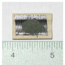
A small amount of the pulverized sample is placed upon a graphite pad that rests upon a ceramic crucible (boat or hearth) and is now ready to be subjected to intense heat of the electric arc.
