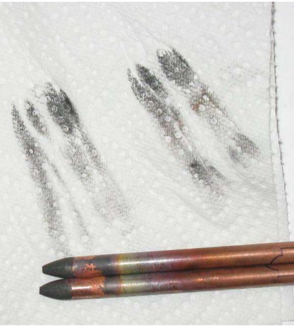
Prior to conducting a Vreeland spectroscope burn the copper-coated carbon arc electrodes are sanded and wiped clean with a paper towel to remove any potential contaminates from previous use.
