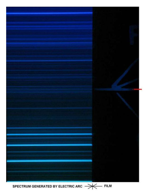
The injected red line at middle right denotes the gold line on film within the blue spectrum. The left film has been edited-out to make this area easier to view.
